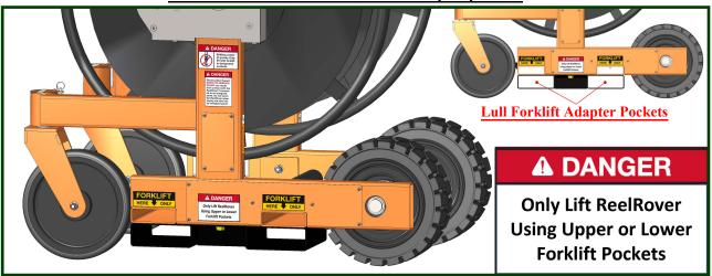
CORRECT LIFTING: Lift all ReelRover<sup>TM</sup> models by positioning the forks being utilized inside the appropriately sized forklift pockets, either located at the bottom of the ReelRover<sup>TM</sup> frame (orange pockets) or within the lull forklift adapter pockets (black pockets) located below the ReelRover<sup>TM</sup> frame, as indicated by the photo above.
